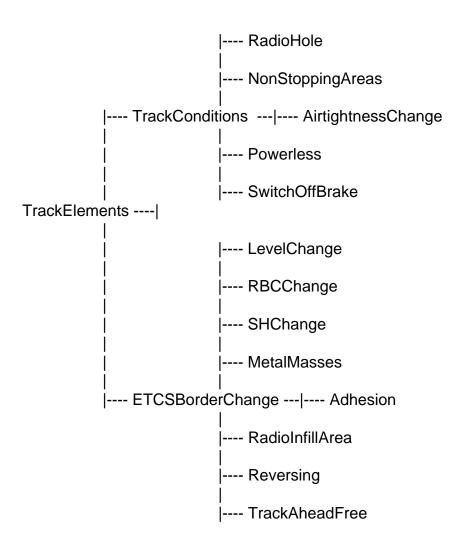
The above described new track elements are classified into two parts. TrackConditions represents common conditions for track elements. ETCSBorderChanges represent special ETCS requirements.
